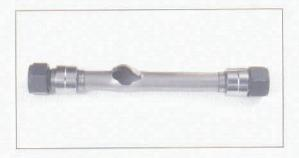
Even after undergoing torsion, fire, stress corrosion, impulse, flexure, and thermal shock testing, the Rynglok tube joints exceed the burst strength of the tubing.
