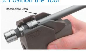
When using the tool in the forward mode as shown, position the tool onto the fitting with the tube side of the ring nested into the moveable jaw. If positioned properly, the front end of the tool will be in the fitting groove. Make sure that the fitting is bottomed into the tool.
