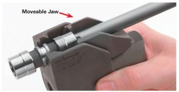
When using the tool in the forward mode as shown, position the tool onto the fitting with the tube side of the ring nested into the moveable jaw. If positioned properly, the front end of the tool will be in the fitting groove. Make sure that the fitting is bottomed into the tool.
