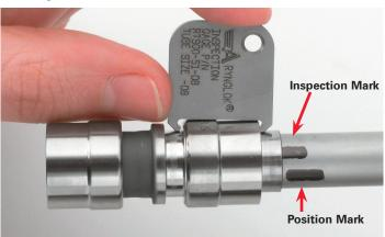
Visually inspect that the ring is fully advanced onto the fitting using the inspection gage. Be sure to verify that the edge of the fitting is within the limits of the inspection mark.
