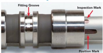
Place the fitting on the tube within the limits of the positioning mark.
