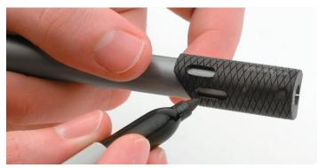
Position the marking gage on the end of the cut tube. Use a suitable marking pen to make the position and inspection marks.
