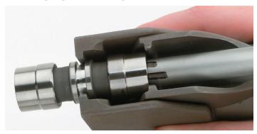
To swage the fitting, apply pressure. Upon completion of swaging, release the pressure, the moveable jaw will return to the original position.
