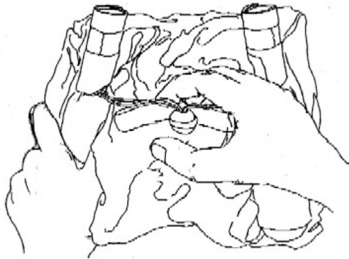
Activating the Essex PBE Oxygen Supply Preparatory to Donning It
