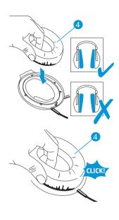
Attach the ear pad 4 so that the side with the thicker padding points downwards as shown.
