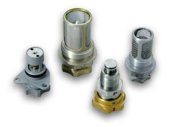
Eaton Tedeco® product line Chip Collectors are the most basic method of detecting wear in lubrication systems. They consist of a magnetic probe and a self-closing valve that allows their removal from a gearbox without draining the oil. The chip collectors are strategically placed in well-designed areas of individual scavenge lines, gearboxes, or other locations to optimize capture efficiency.
