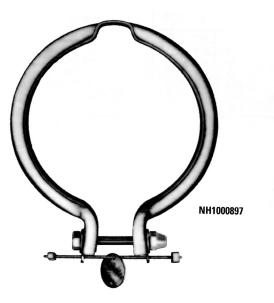
Eaton's Aeroquip one-piece, thermal expansion adaptable clamp is now being used on a number of Cessna and Piper aircraft as an exhaust connection. The high apex and spring design lugs were specifically designed to accommodate thermal expansion caused by high temperature differential between hot internal exhaust gas and cooler ambient temperatures. The one-piece design eliminates welds or
