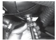
2. Take hold of the knurled nut and with a combination pushtwist motion, open the valve.
