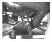
Simply remove the plug from the bottom of the oil sump and install the drain valve in the port. Wrench torque carefully. Safety wire valve to sump.
