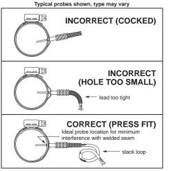
Figure1. Welded Boss Type
